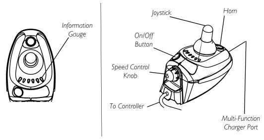
FIGURE 5.1 SPJ™ Joystick Switches and Indicators
